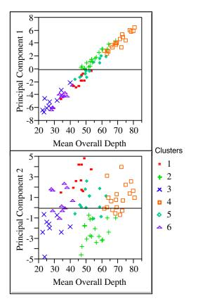
Figure 3. Principal components 1 and 2 as a function of mean overall depth rating and cluster.
